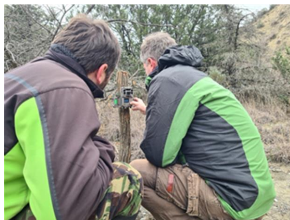
Photo #1. Installing a camera trap on a wooden post
